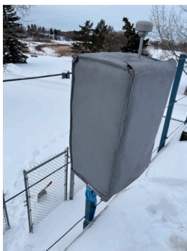
Figure 1: The Dust Sentry deployed at the Henry Pirker station, showing the winterization jacket.
